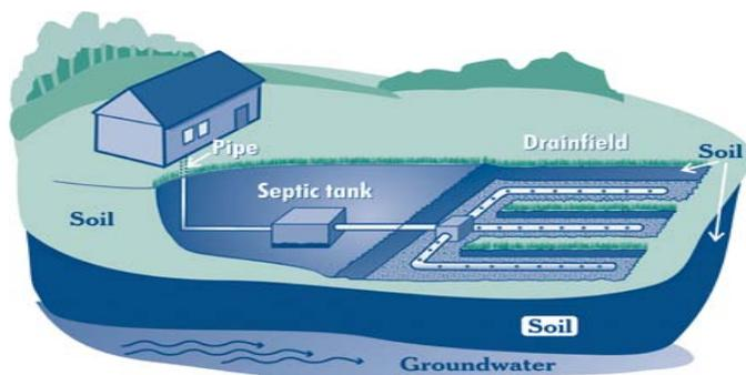
The septic tank also allows large materials to settle to the bottom of the tank. Scum and grease will float on the top of the wastewater. The dissolved organic material in the wastewater is allowed to flow out of the tank by a pipe and through a distribution box into several pipes that lead to the dispersal system (also called lateral field, drainfield or leachfield). This configuration is defined as a **conventional onsite sewage system (COSS)**.
